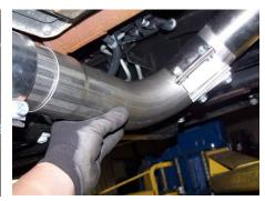
• Install y-pipe outlet extension and bolt to back half of exhaust and band clamp it to the back of the y-pipe. Snug the band clamp but do not fully tighten.
